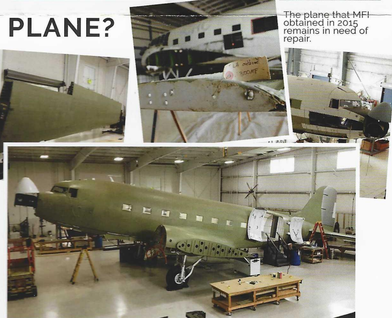
Pictured above is the proposed fuselage and center section that have already been refurbished and would have our completed wings attached.
